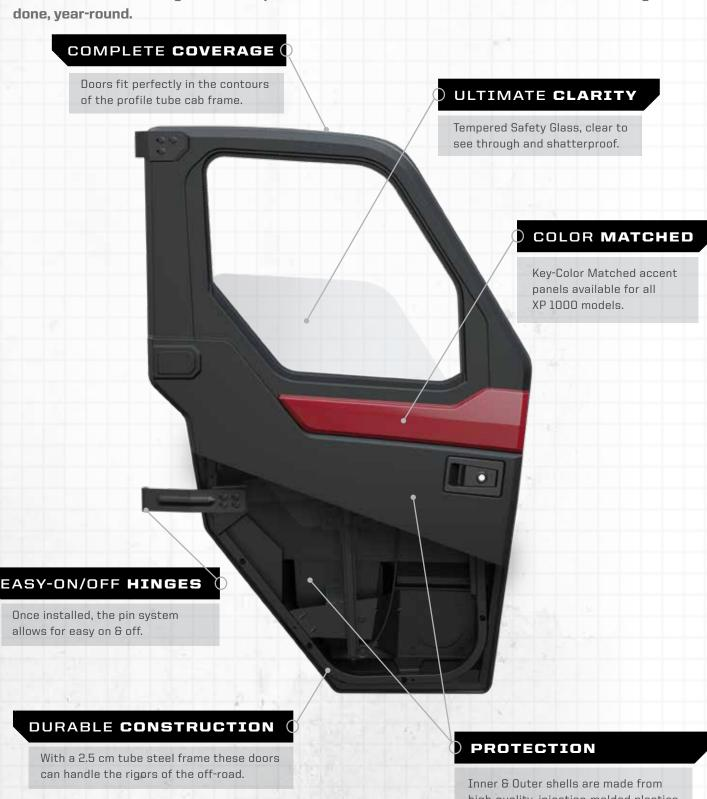
Inner & Outer shells are made from high-quality, injection-molded plastics using a state-of the art process to shield from the elements and more.
